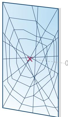
a) Numerous fractures inside the sample are acceptable, except for a chipping or a hole whose diameter is sufficient for a 76 mm ball to pass through, after applying the maximum force of 25 N. Moreover, if pieces come apart three minutes after the impact, their total weight should not be greater than the equivalent weight corresponding to 10 000 mm<sup>2</sup> of the original sample.
