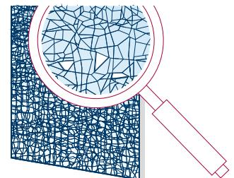
Fracture pattern of toughened glass ESG
