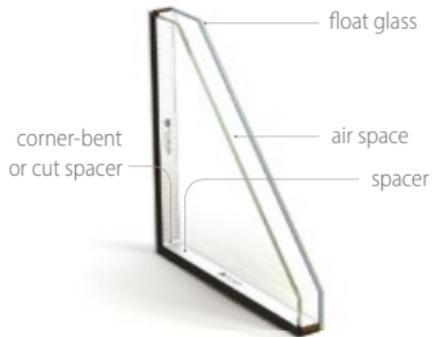
First modern tight IGUs were developed in 1950s, but they started to be produced and used commonly in buildings about 20 years later. The technology owes its development to the deficit in generation of thermal energy to heat buildings.
