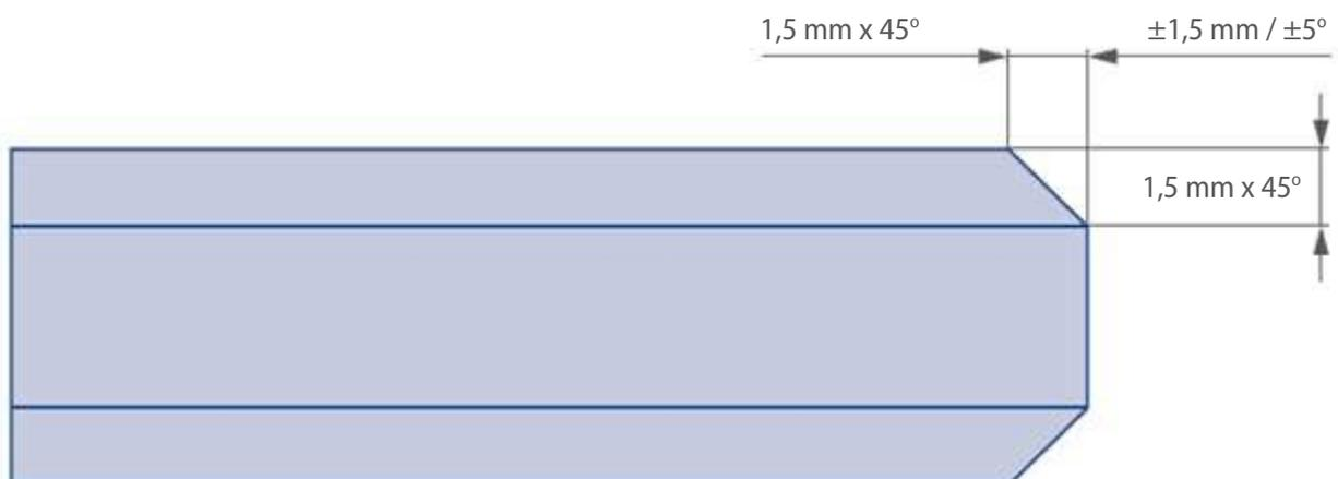
Fig. 4 Diagram of ground or polished glass edge
