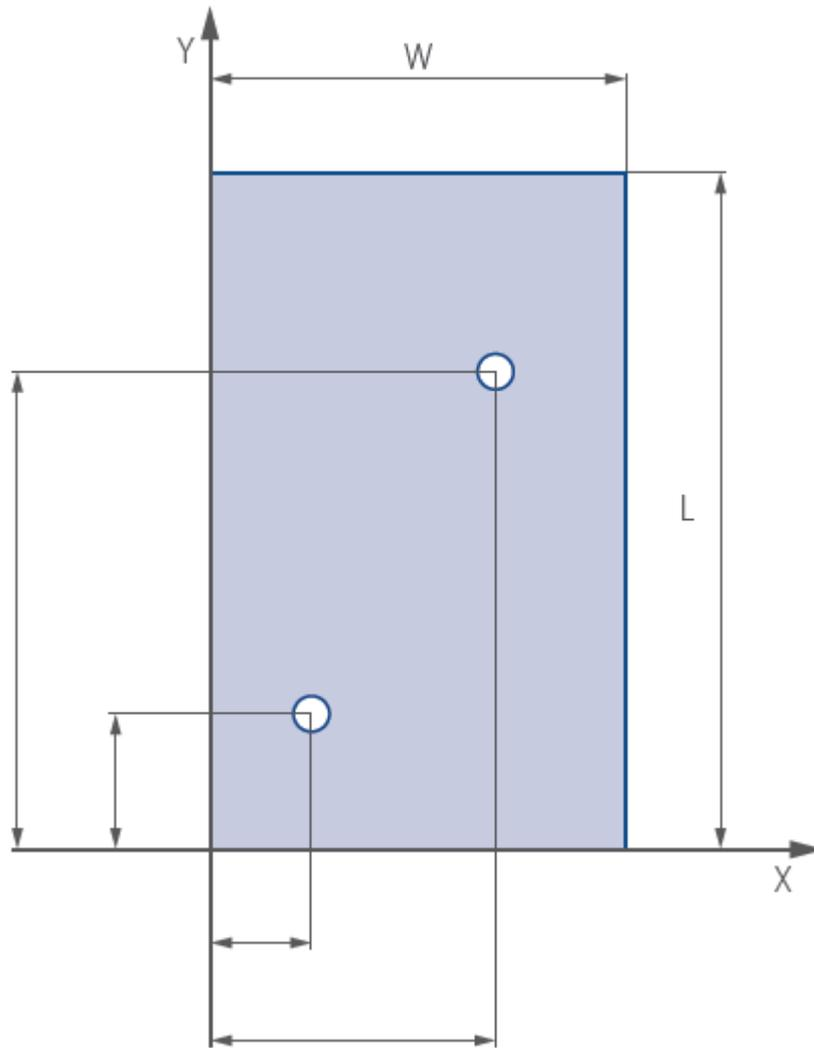
Fig. 17 Measurement of hole locations on the glass
