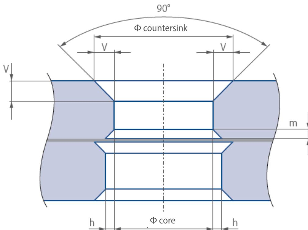
Fig. 35 Diagram of holes in laminated glass,  $h = 2 \text{ mm}$ ,  $m \geq 1.5 \text{ mm}$ ,  $v = (\varphi_{\text{chamfer}} - \varphi_{\text{core}}) / 2$
