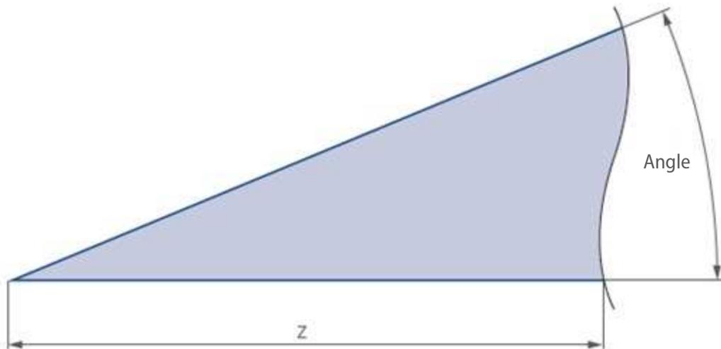
Fig. 1 Sample sharp corner of glass with cut-out area marked, with a length of z
