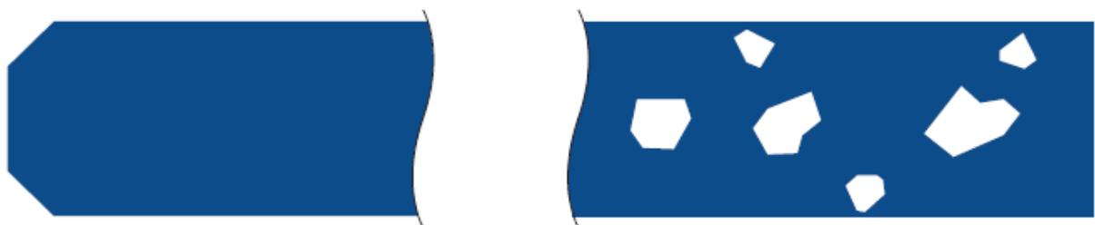
Fig. 7 Ground periphery (with shiny areas) – arrised edge with trimmed face or ground edge
