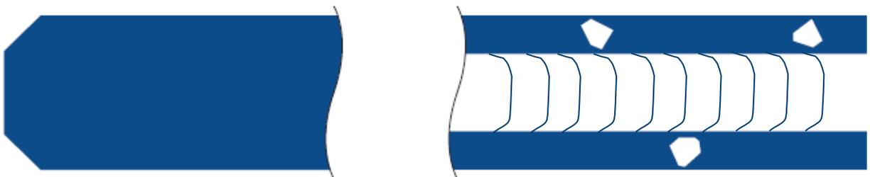
Fig. 6 Machined periphery (with shiny areas) – arrised edge
