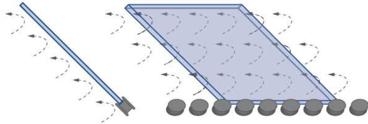
Fig. 25 Diagram of the PREMIUM TOUGHENED tempering process
