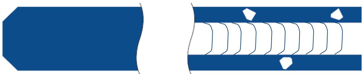
Fig. 2 Arrised edge diagram
