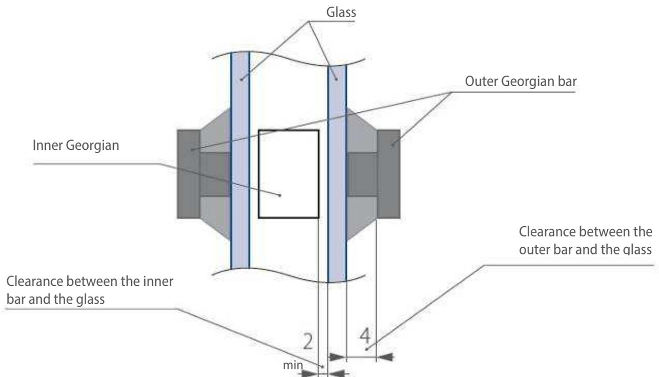
Fig. 2 Installation of inner and outer Georgian bars
