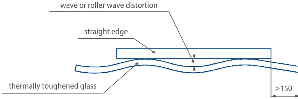
b) Measurement of wave or roller wave distortion
