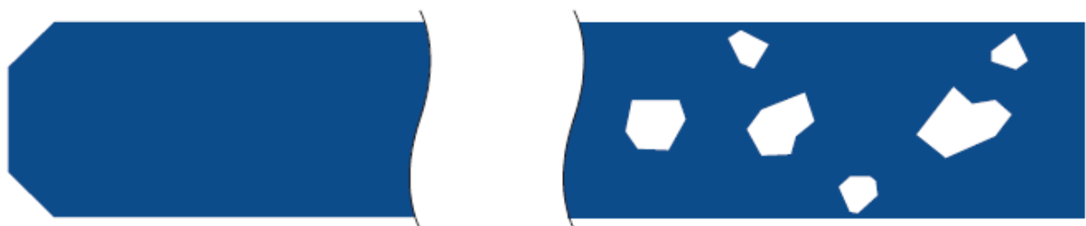
Fig. 7 Ground periphery (with shiny areas) – arrised edge with trimmed face or ground edge
