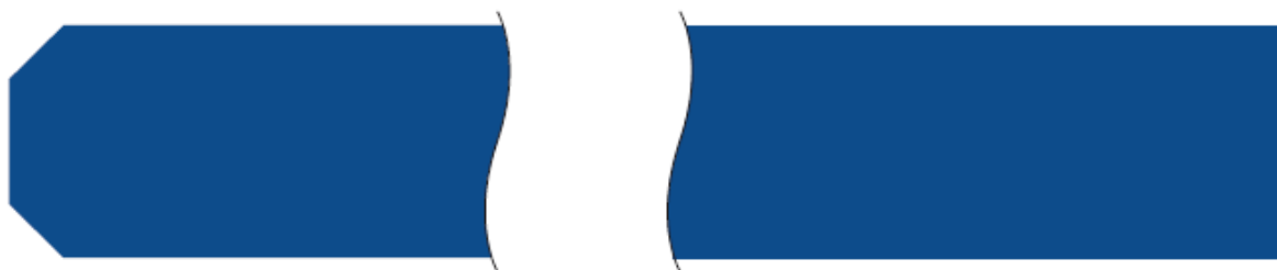
Fig. 8 Smoothed ground periphery (no shiny areas) – ground edge
