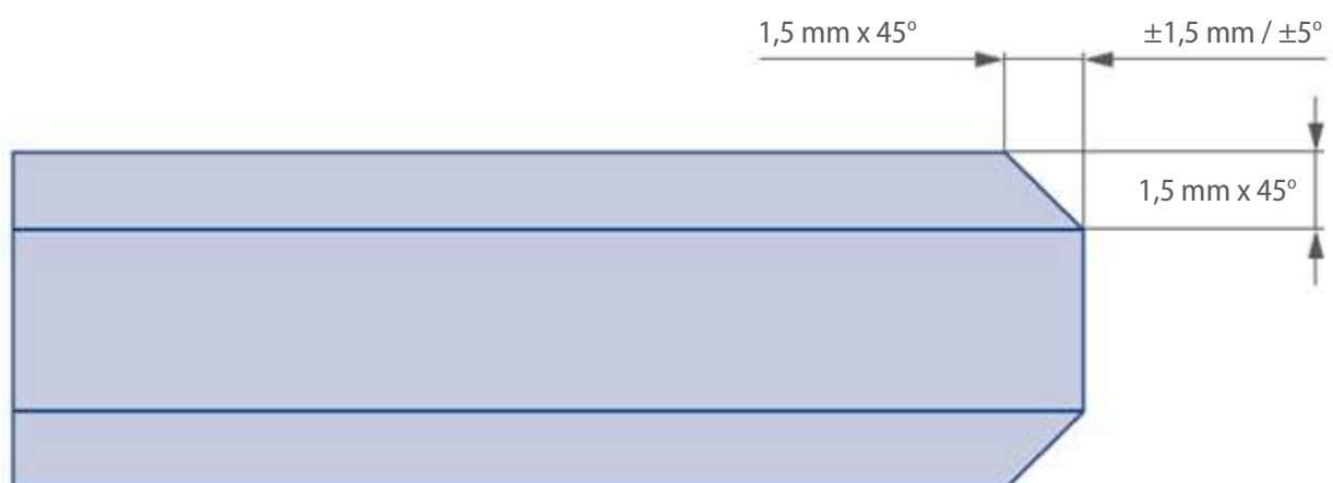
Fig. 4 Diagram of ground or polished glass edge
