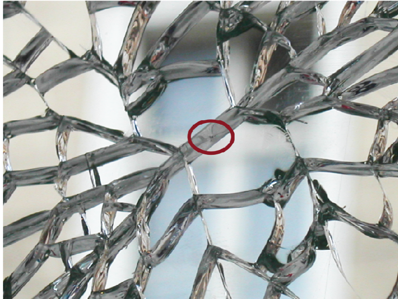
Fig. 30. Example of spontaneous cracked glass due to the presence of nickel sulphide
